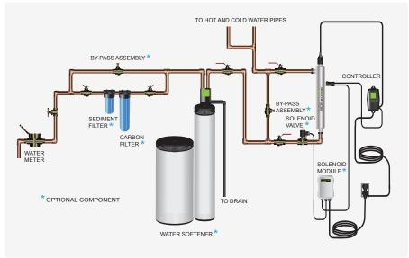
Figure 1. Recommended POE Installation Location
