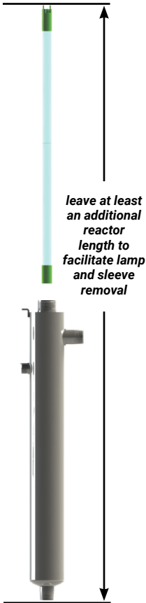
Figure 2. Lamp Removal Spacing
