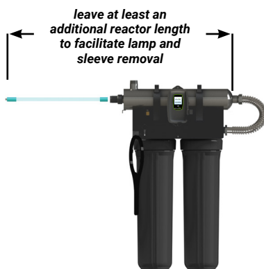
Figure 3. Lamp Removal Spacing
