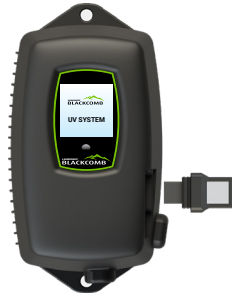
Figure 10. Lamp Key Installation
